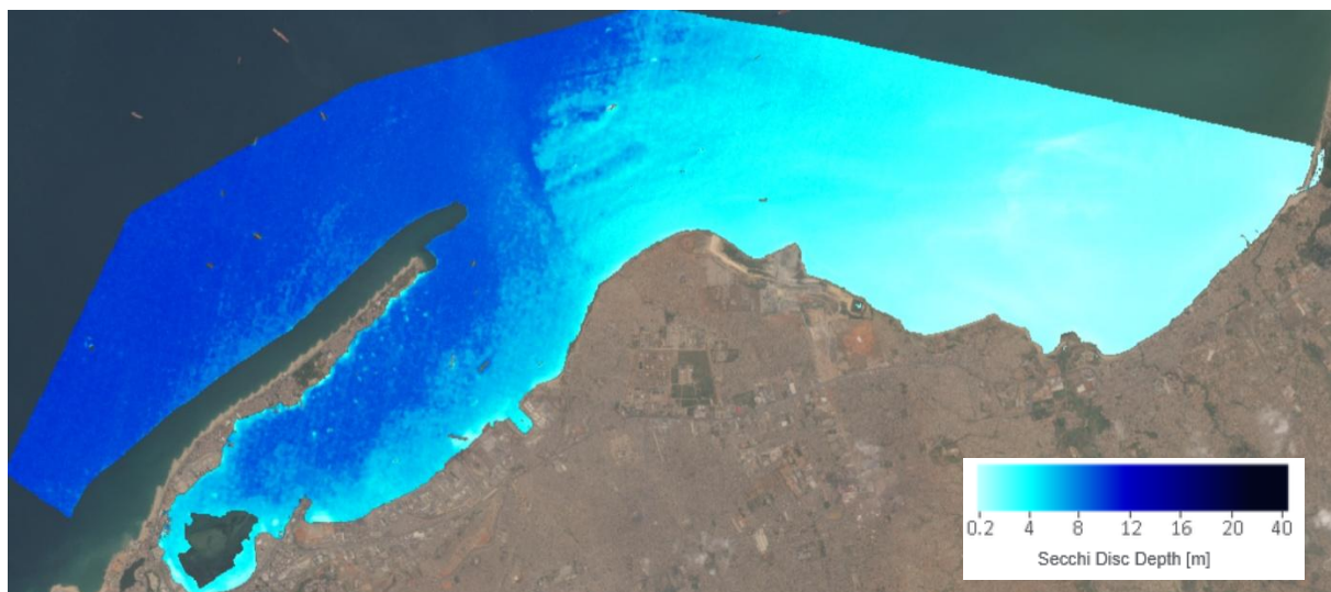
Figure 13: Secchi Depth map showing the visibility on 3 rd July 2026 – the scene shows good visibility at Luanda Beach, medium visibility in the Luanda Bay and low visibility in the Eastern part of Luanda
