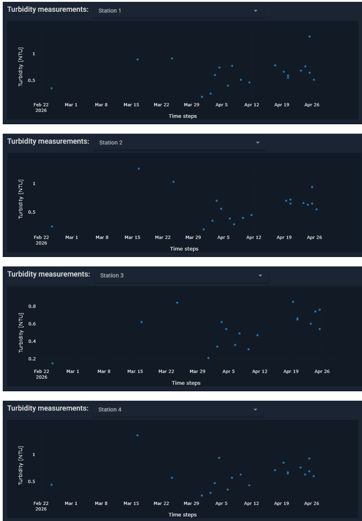
Figure 12: Turbidity measurements at 4 points in the actual race location. The order of panels follows following order from top to bottom: Station 1, Station 2, Station 3, Station 4
